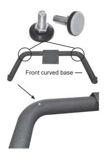
**2.** Locate the threaded inserts on the underside of the front curved U base at the sections that curve.
