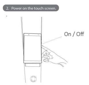
The power switch is on the right side of the touch screen. Press and hold it for 5 seconds
