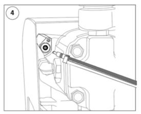
While holding both together, guide end of power cord into barrell jack. Push firmly to make connection.
