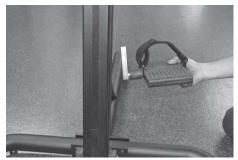
**15.** Attach foot pedals with "L" shape bracket pointing up, using (2) 3/8" x  $1 \frac{1}{2}$ " long hex head bolts.
