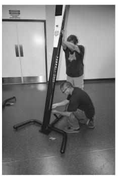
**11.** Attach tubular brace between main post and back tubular floor base with (2) 3/8" lock nuts **DO NOT TIGHTEN FULLY AT THIS TIME.**
