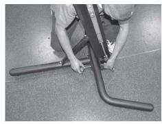
**10.** Attach back tubular floor brace to post with (2) hex head bolts 3/8" x 3¾" long and (2) lock nuts. **DO NOT TIGHTEN FULLY AT THIS TIME.**
