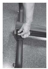
**7.** Screw in (4) self tightening base bolts.
