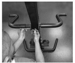
**18.** Insert 3" long spacer and FULLY TIGHTEN all 3 bolts and nuts.
