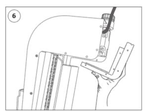
When power cord plugged in and secured, attach back cover while guiding wire up and through reservoir clearance hole in housing.
