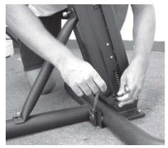
**12.** After tubular brace is in place, go back and **FULLY TIGHTEN** the (2) 3 ¾" long base bolts.
