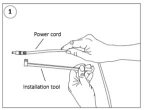
Align end of power cord plug with installation tool.
