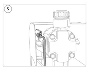
Using tool plug in power cord into barrell port.
