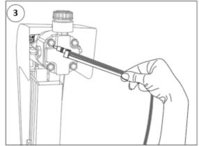
Using a light source, locate barrell jack which is accessed on the backside, top of unit.
