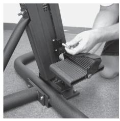
Attach foot pedals with "L" shape bracket pointing up, using (2) 3/8" x 11/2" long hex head bolts.
