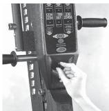
Clockwise rotation of the control knob, (to the right), slows the rate of motion (easier). Counterclockwise rotation of the control knob, (to the left), increases the rate of motion (harder). The rate of motion, (slower/faster), may be
