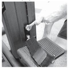
Securely **TIGHTEN** foot pedals with 9/16" wrench.
