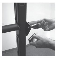
Insert 25/8" long spacer and **FULLY TIGHTEN** ALL three bolts and nuts with 9/16" wrench.
