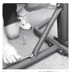
Next, tighten the <u>BOTTOM</u> lock nut on the back brace to complete post assembly.
