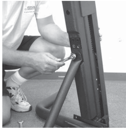
Then go back and TIGHTEN FULLY the TOP lock nut on the tubular brace.
