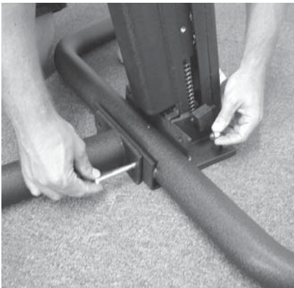
Attach back tubular floor brace to post with two hex head bolts, 3/8" x 33/4" long. (2) 3/8" lock nuts. DO NOT TIGHTEN FULLY AT THIS TIME.
