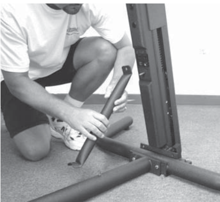
Attach tubular brace between post and back tubular floor base with (2) 3/8" lock nuts. DO NOT TIGHTEN FULLY.
